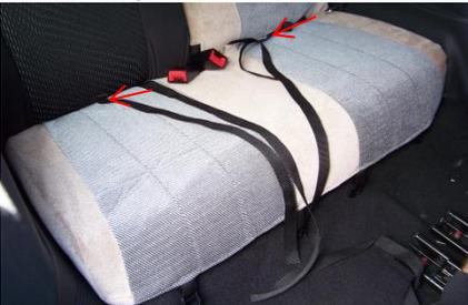
Place the cover on the cushion, matching its contours and cutouts. Tuck in the top of the cover pushing the straps towards the back of the cushion.
