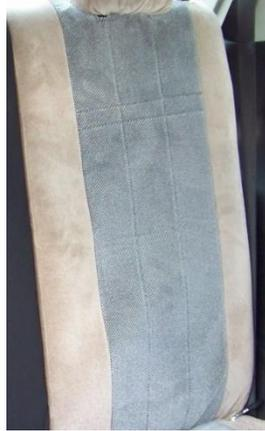
Pull on the strap on the side of the backrest to pull the backrest forward. Place cover over the backrest, matching its contours and cutouts. Tuck in the bottom of the cover towards the back sticking the velcro to the carpet ; also tuck in the "X"
