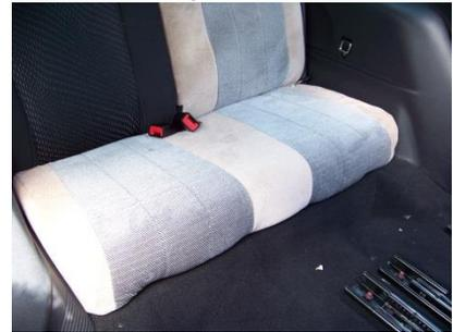
Pull on the straps to fit the cover to the cushion, once it's nicely fitted but the cushion back on its mounts.
