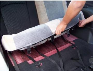
Pull up on the front of the cushion, releasing it from its mount. Pull the straps from underneath and buckle them accordingly.
