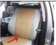
Step#2 – Install Backrest Part 1\* (Slip the cover onto the backrest and tuck in the flaps.)
