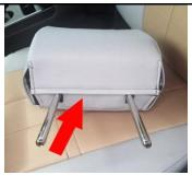
Step#1 - Remove Headrest (Remove and Apply the headrest cover, attach the Velcro on bottom.)
