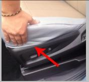
Step#4- Install Bottom Cushion (Tuck in the remainder of the fabric in between the plastic)
