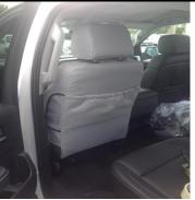
Step#3 – Install Backrest Part 2\* (Attach the Velcro and straps together on the back of the seat)
